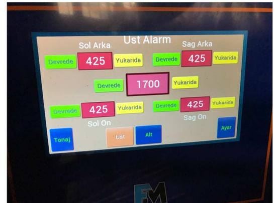
It is possible to work longer periods without urgent maintenance by avoiding press overload damages. Keeping the press forces within recommended limits prevents emergency stops and improves the die life.
